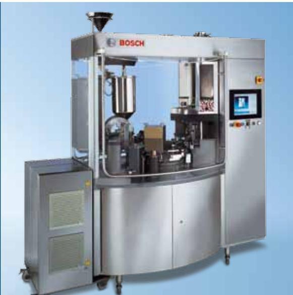
The **GKF 1400 L** is equipped with a servo-driven liquid pump that allows for continuous fill level control and an optional drip-retract function. All machine settings can be controlled via the user-friendly touch-screen HMI.
