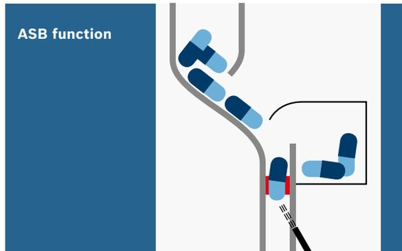
The mechanical capsule cap scanner determines if there are blockages in the empty capsule infeed. A repeated missing capsule in a particular segment bore is recognized by the consecutive fault function. Deformed capsules in the capsule magazine are blown out via individual compressed air lines and routed to a separate deformed capsule container.
