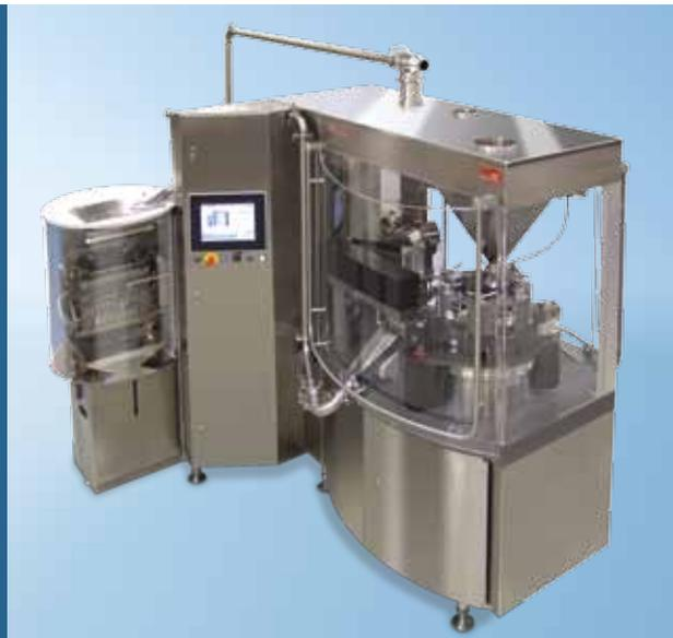
The **GKF 1400 ASB 100%** is equipped with an integrated checkweigher. Every capsule produced on the capsule filler is individually and precisely weighed. Only capsules with a weight within the pre-set tolerances are accepted and made into the good capsule container. Overweight and underweight capsules are removed and separated into the bad capsule container.
